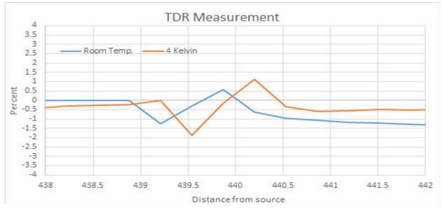
Typical performance of a 40GHz Cryogenic Attenuator \*Testing done by a 3rd party lab
